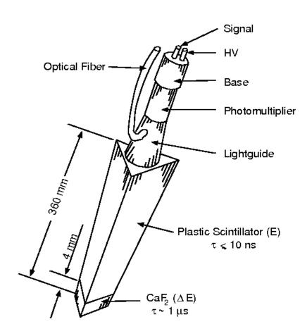
Plastic ball covered 30< $\theta$ <160°. It consisted of 655 detectors. Particle ID via  $\Delta$ E-E.
