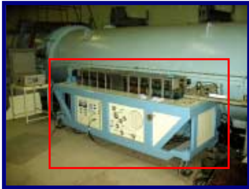
IHEP laser (CO 2 , 2.7 J, 10 μm, 0.25 Hz)
