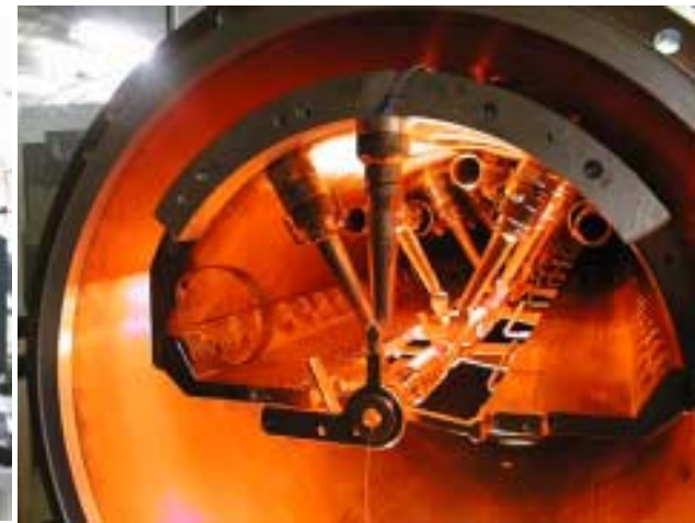
Sector H-cavity of "Ural" RFQ DTL (prototype)
